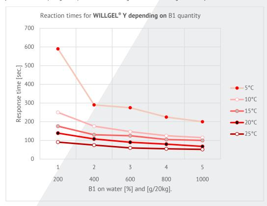
It is also possible to increase the amount of water on both sides (A and B) by a <u>maximum of 50% to</u> obtain longer reaction times and an even lower viscosity. The final product is then weaker, but still has sufficient soil consolidation properties.
